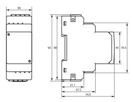
Figure: Dimension diagram (in mm)
