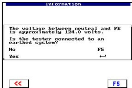
If the test system is used other than for the intended purpose, i.e. in an IT system, the measured values of any leakage currents will not be reproducible. The test result cannot be used. Disconnect the test system and connect it to an earthed socket outlet.
