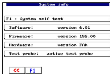
Once you have pressed "F1: System self test" you can choose between an internal self test and a more extensive test with the TB3 test box.
