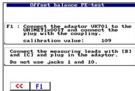
Zero balancing takes approximately 5 seconds to complete. The calibration value is saved and is retained until a new zero balancing procedure is performed for this measuring path.
