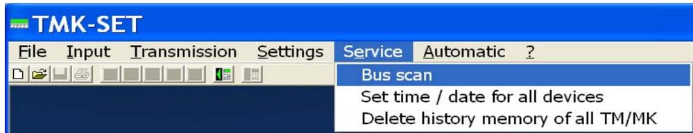
The "Bus scan" function is used to scan the entire BMS network. All detected devices are displayed including their device addresses and version numbers. This overview makes the programming process easy. You can also use this function to check that all devices have been connected correctly and their bus addresses have been set correctly.
