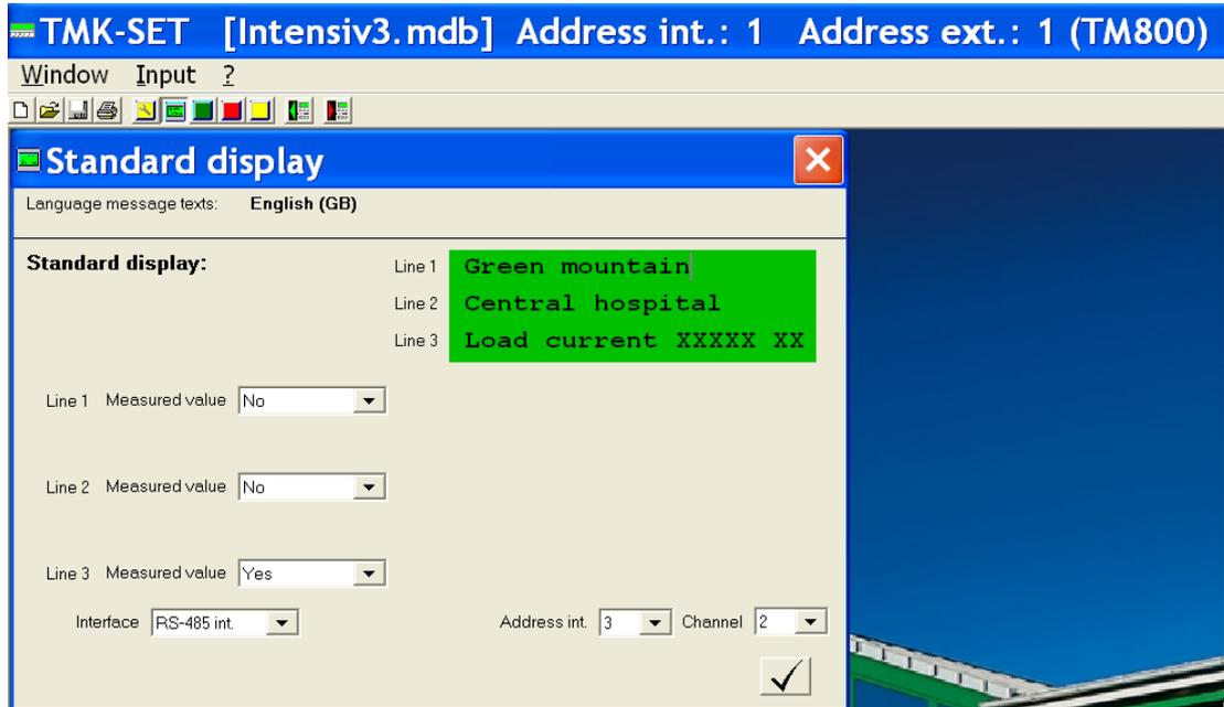
1. Enter the text that is to be displayed on the first three lines of the display during normal, fault-free operation.
