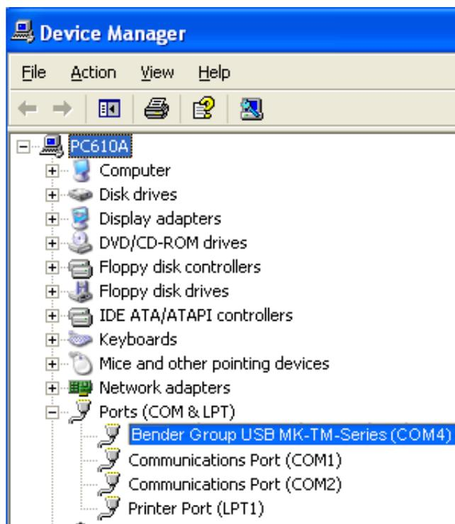
If necessary, you can assign a different number to the COM interface. Right-click on "Bender TMK USB Port (COM\_)" and select "Properties". Enter the desired COM port number under "Port Settings -> Advanced" (allowed range up to COM16).
