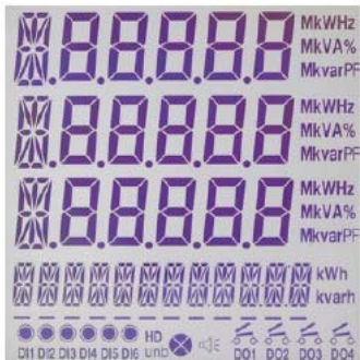
Abb. 6.2: Display during an LCD test
