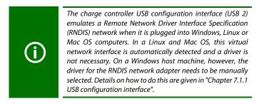
The charge controller uses the local IP address **192.168.123.123** with a subnet mask of 255.255.255.0 on the virtual network interface corresponding to the USB configuration interface. The PC (or target) is automatically assigned a corresponding IP address via the Dynamic Host Configuration protocol (DHCP) once it is connected and communication with the charge point is based on this IP address.
