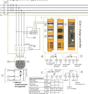
Charge point with type 2 socket:
